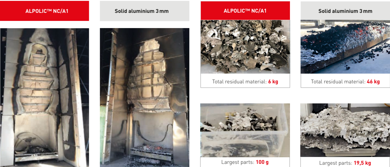
Result after a large-scale fire test (BS8414-2)
