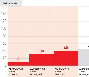
\*Comparison of debris quantity in KG during BS8414 large s cale f ire tests with different cladding materials.
