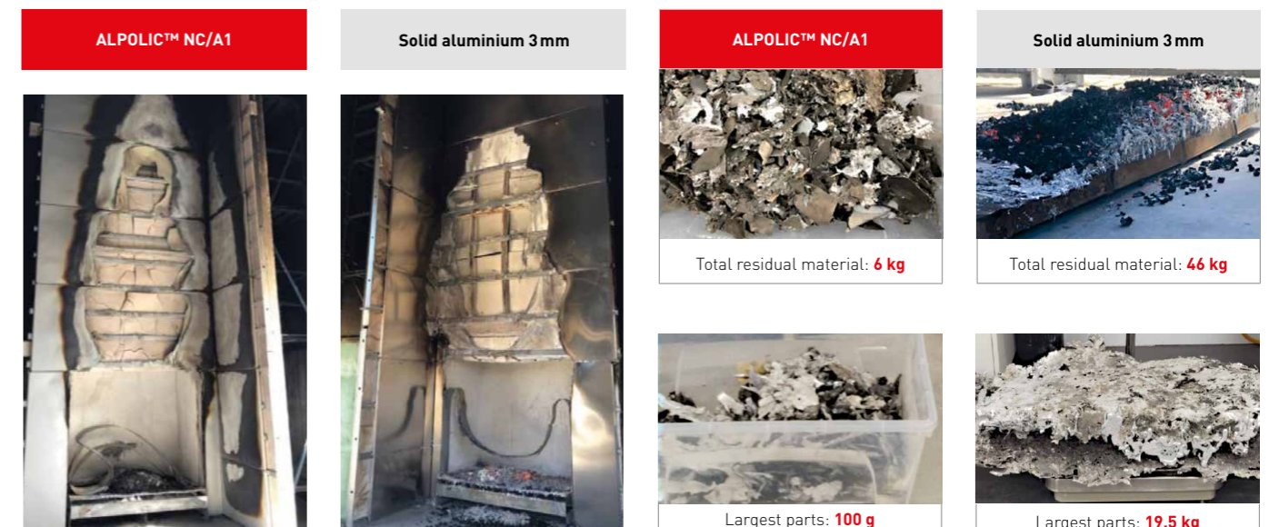
Result after a large-scale fire test (BS8414-2)
